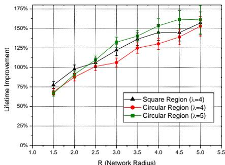
Fig. 12. Average lifetime improvement for networks with one mobile over the static network (confidence interval 95%). For the square network, the sink is put at the center of the square and the network radius  $R$  is defined as half the side length of the square.
