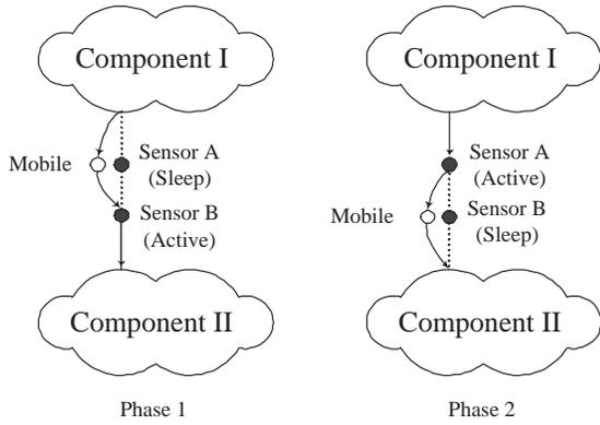
Fig. 1. One mobile relay can take over the tasks of *multiple* bottleneck nodes (sensor A and B) during different network time periods.
