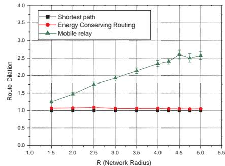
Fig. 13. Comparing the route dilation for different approaches. (Network on square area with  $\lambda = 4$ , confidence interval 95%)
