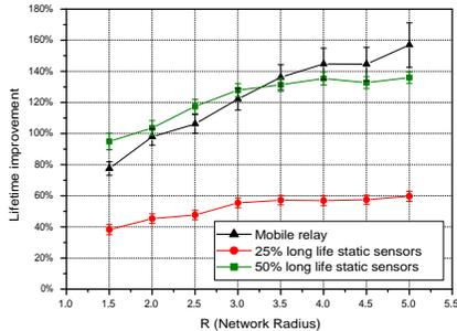
Fig. 15. Comparing the lifetime improvement of adding one mobile relay with solutions that add more energy to static sensors. (Network on square area with  $\lambda = 4$ , confidence interval 95%.)
