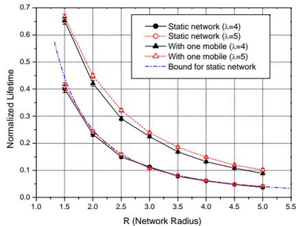
Fig. 11. Network lifetime for nodes randomly deployed on a circular region, for  $\lambda = 4$  and 5 (confidence interval 95%)
