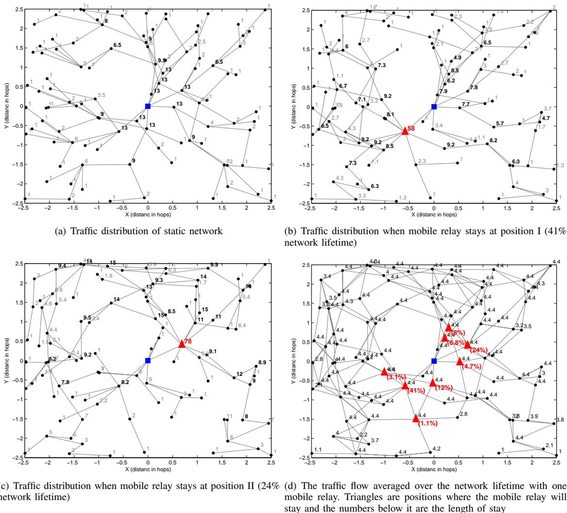
Fig. 10. Traffic flow in network with 100 sensors in  $5 \times 5$  square area. The sink is marked as the square in the center of the network. Mobile relay is marked as triangle. In this example, we only show two positions and the corresponding traffic flow, there are actually 8 positions at which the mobile relay will stay during the network lifetime.
