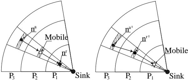
Fig. 4. Aggregation node selection and the relay path construction
