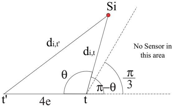
Fig. 2. Sensor  $S_i$  can detect both point  $t$  and  $t'$ , but cannot distinguish them.
