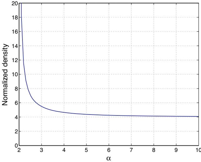
Fig. 4. The relationship between network resolution and sensor density.  $\alpha$  is network resolution divided by  $e$ , the distance measurement error. The normalized density is ratio of localization coverage compared to detection coverage.
