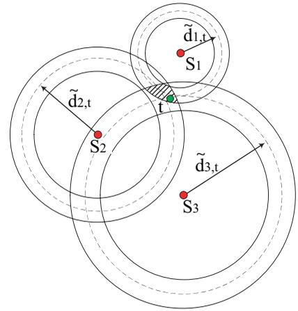
Fig. 1. Each of the three sensors  $S_1$ ,  $S_2$  and  $S_3$  can provide distance information of the target at point  $t$ . The target location will be within the intersection of the annuli around them, shown as the shaded area.
