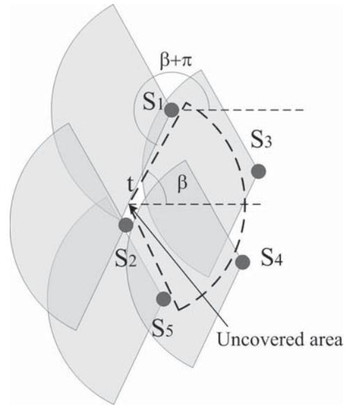
Fig. 7. Sector coverage for a given orientation of  $\beta$ .
