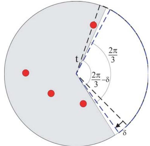
Fig. 8. Increasing  $\beta$  by step size of  $\delta$ . The void is two opposite sectors of  $(r, \frac{2\pi}{3})$ , as the two white sector in the figure. The sensing region is the dotted sectors, which is  $(r, \frac{2\pi}{3} - \delta)$ .
