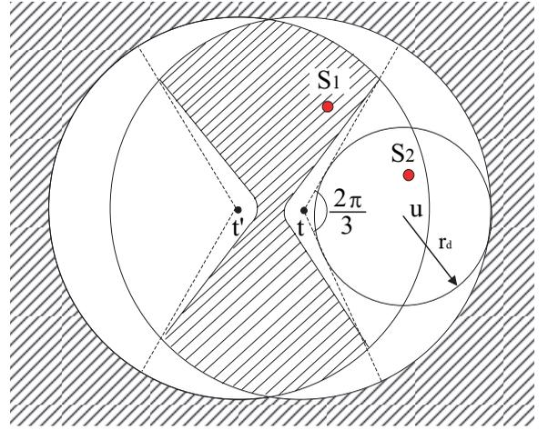
Fig. 3. Sensors in the shaded area, such as  $S_1$ , cannot distinguish the point  $t$  from  $t'$ . Sensors in the white area, such as  $S_2$ , can distinguish these two points, so there should not be any sensor in the white area.
