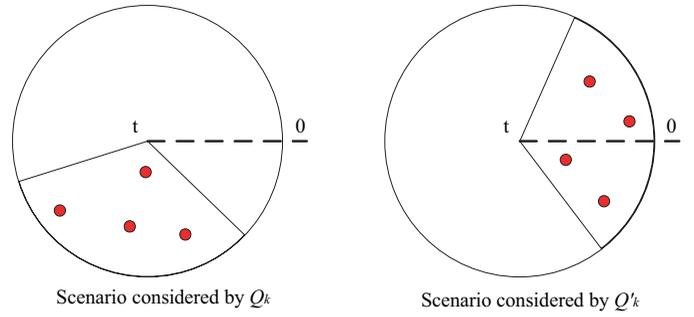
Fig. 5. Bounding the probability that there exists a sector void of  $(r, \frac{2\pi}{3})$ , two scenarios are considered based on whether the sector crosses the zero angle.
