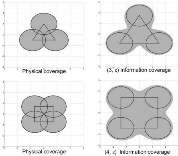
Fig. 1. Comparison of physical and information coverage for regular sensor deployment ( $\alpha = 1.0$ ,  $\epsilon = 0.683$ ).
